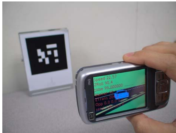
Figure 1. ID-encoded ARToolkitPlus marker used for computing the pose of the mobile device in 3D space.
